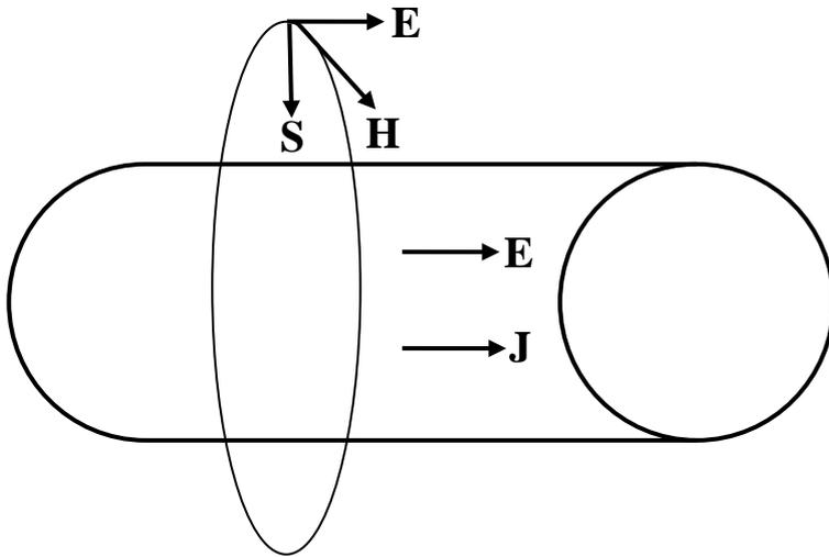
Fig. 4. Poynting vector in a resistive, current carrying wire. Redrawn based on [2].
