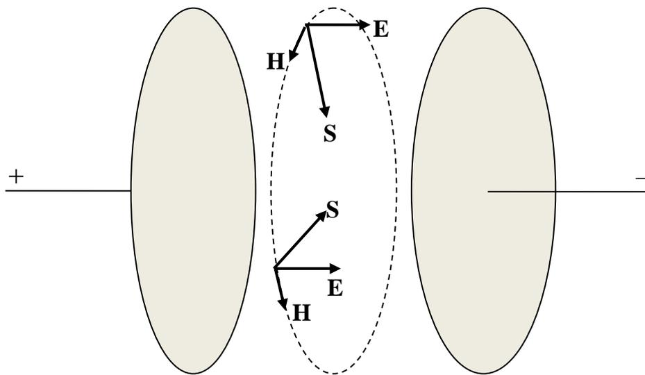
Fig. 3. Poynting vector in a charging capacitor. Redrawn based on [2].
