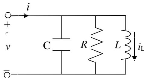
Fig. 1. An electric circuit in which the input power is conserved as stored energies in  $C$  and  $L$  and as heat energy in  $R$ .
