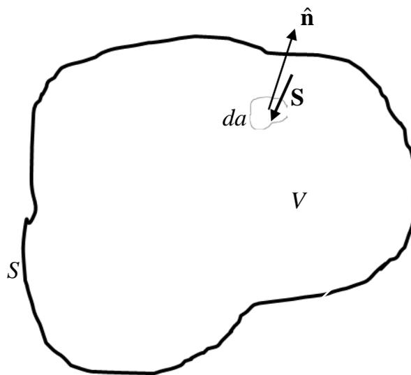
Fig. 2. Electromagnetic power flow into volume  $V$  through surface  $S$ .
