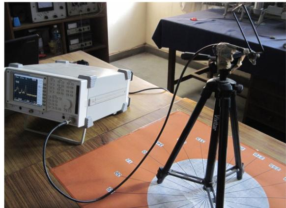
Fig. 8 Photograph of Test set up of square loop antenna with spectrum analyzer.
