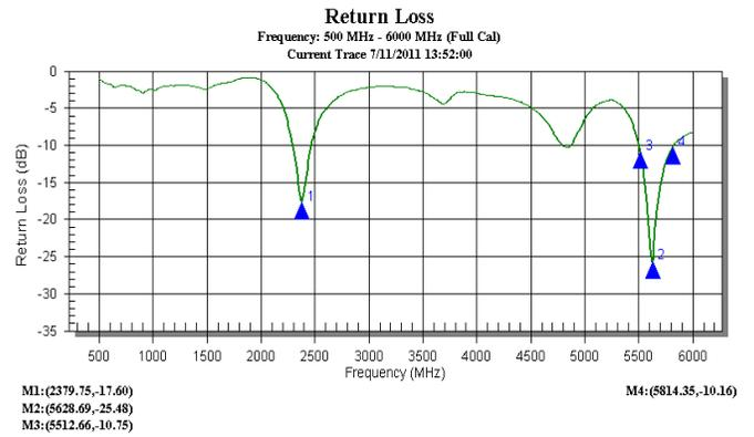
Fig.13 Return loss ( $S_{11}$ ) characteristics of collinear microstrip patch
