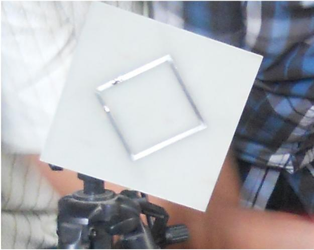
Fig.10 Photograph of microstrip patch blade antenna at test set up.
