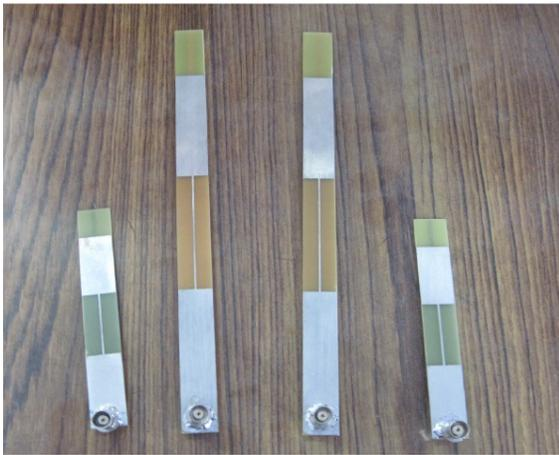
Fig. 4 Photograph of fabricated microstrip collinear antenna
