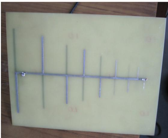
Fig. 5 Photograph of fabricated microstrip log periodic antenna.
