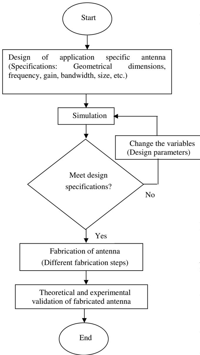
Fig. 3. Flow diagram to design, fabricate and test the assigned antenna.
