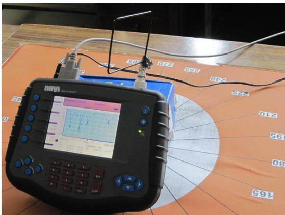
Fig. 6 Photograph of fabricated wired square loop antenna with site analyzer.
