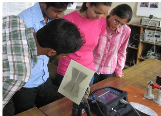
Fig.9 Photograph of group of students with test and measurement set up for microstrip bow-tie antenna.
