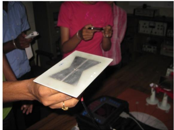
Fig.7 Photograph of test set up for microstrip bow-tie antenna.
