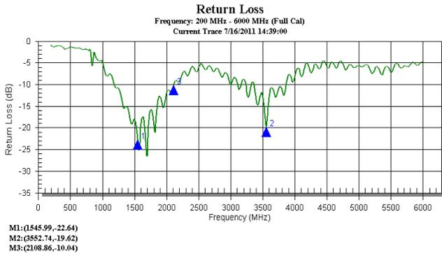
Fig. 11 Return loss ( $S_{11}$ ) characteristics of Bat wing antenna.
