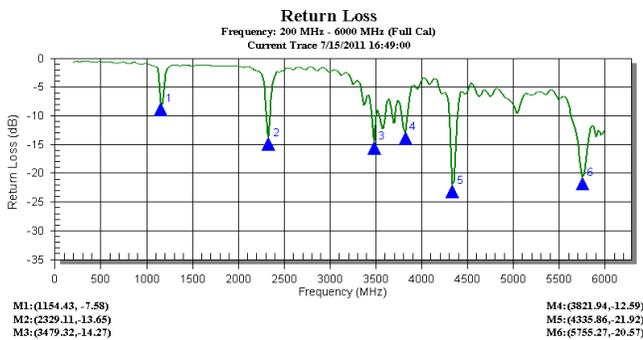
Fig.12 Return loss ( $S_{11}$ ) characteristics of stacked rectangular microstrip patch antenna.
