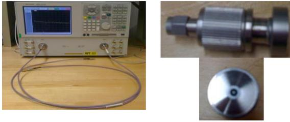
Figure 7 Agilent 85070E dielectric probe kit
