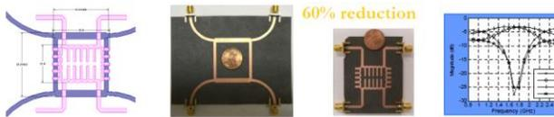
Figure 12 Microstrip Quadrature Hybrid with Artificial Transmission Lines (ATL) with 60% size reduction
