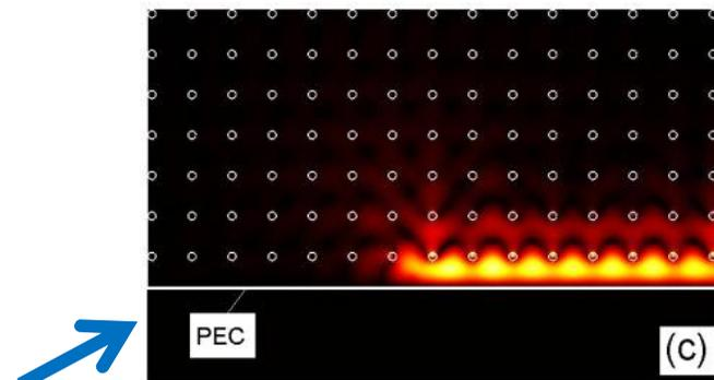
*One-way transmission associated with edge state*
