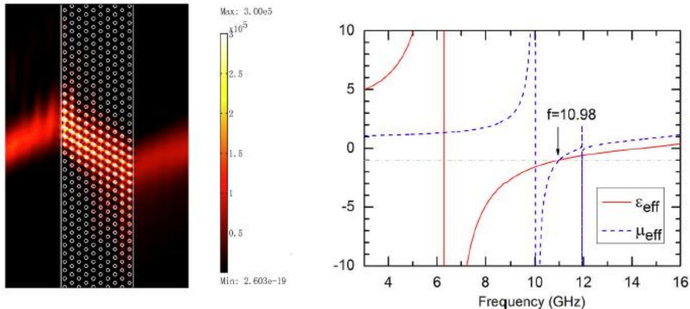
*A beam of Gaussian wave incidences obliquely on the boundary of MPC of hexagonal lattice. It refracts negatively on both sides of the MPC at 10.9 GHz
