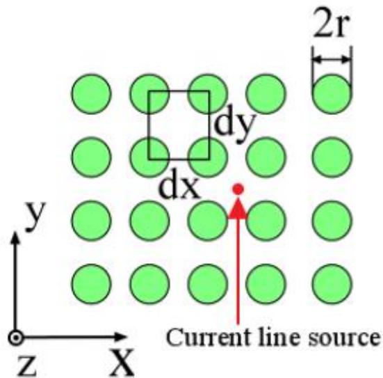
*The antenna consists of magnetic rods and a line current line source embedded in. The rods are in diameter of 4 mm and made of ferrite YIG with saturation magnetization  $4\pi M_s = 2200$  Ga and permittivity  $\epsilon_r = 12.2(1 - j 0.006)$*
