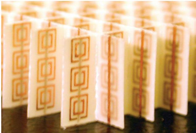
*Metamaterials of which the feature size is much smaller than wavelength*
