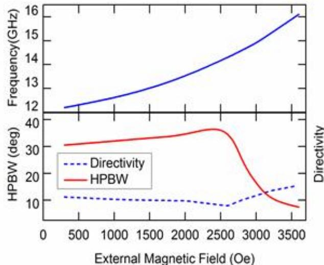
The operating frequency moves from 12.2 to 14.3 GHz (about 2 GHz) when bias field changes from 300 to 2600 Oe. The average directivity in the tunable range is about 32.
