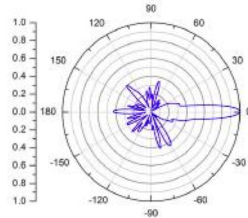
With the rod array, we designed the LHM-antenna which achieves the directivity and HPBW about 12.2 and 12°, respectively.
