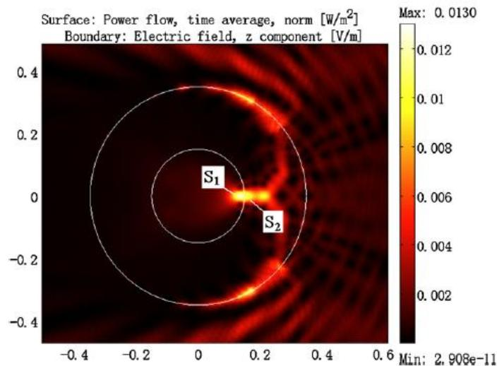
*Power flow distribution for the LHM shell illuminated by a plane wave incident from right-hand side.*
