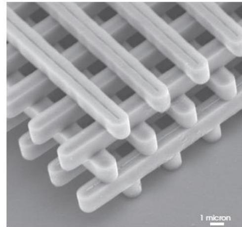
*EBGs structure of which the feature size is the same order of wavelength*
