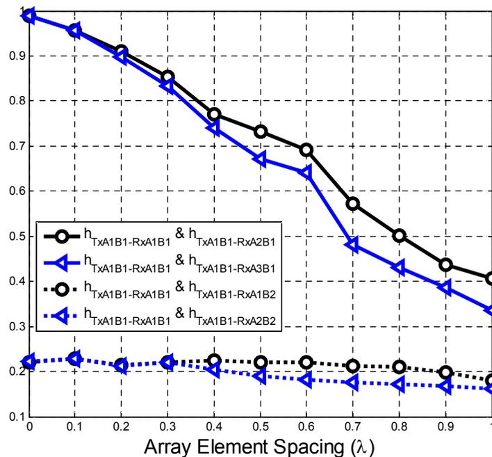
Fig.2. Correlation coefficient versus Rx array element spacing.
