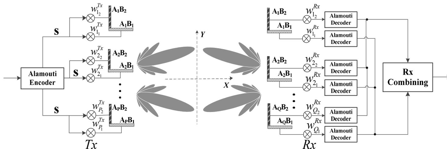
Fig.3. The proposed MIMO transceiver to accommodate Alamouti code and beamforming technologies simultaneously.
