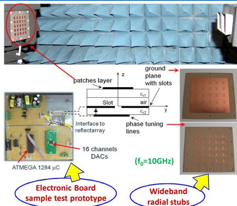
Electronic Board sample test prototype
