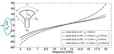
Simulated input reactance vs. frequency for different stubs
