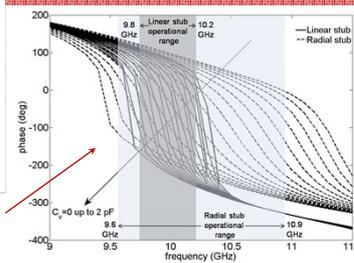
Simulated phase curves vs. frequency for different diode capacitance values (Comparison between two cells respectively driven by a radial and a linear phasing line)
