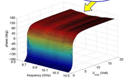
Measured phase curves vs. frequency and varactor bias voltage
