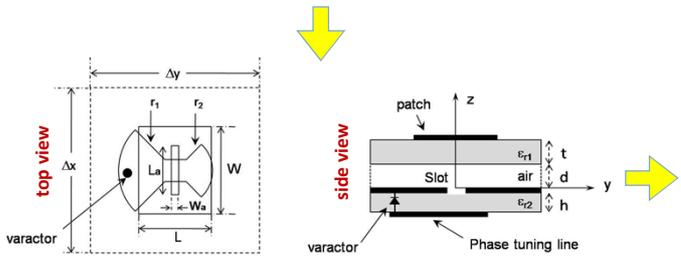
This novel phasing line geometry **improves the reconfigurability frequency range of the cell** due to the fact that the **input impedance of a radial stub has a smoother behavior** with respect to an equivalent linear stub.
