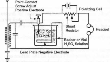
**Figure 1** An early version of Fessenden’s spark gap telegraphy transmitter a); and b) Fessenden’s receiver employing an electrolytic detector.
