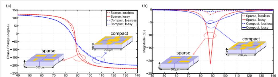
Simulated reflection coefficients for 2D uniform infinite interlaced triangular-lattice dipole arrays with compact (blue dash and solid lines) and sparse (red dash and solid lines) configurations.
