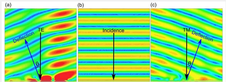
Instantaneous scattered field from the reflectarray with lossless substrate at 1 THz. When the incident wave (b) is normal to the surface of the reflectarray, the TE and TM polarized wave are deflected into two different directions with the designed angles shown in (a) and (c), respectively.
