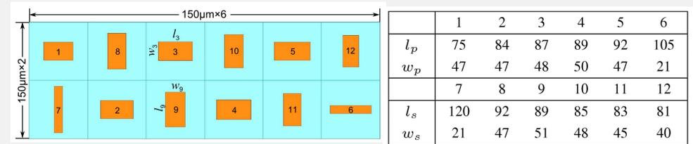
Layout of a subarray made of 12 dipoles and the dimensions of each dipole.
