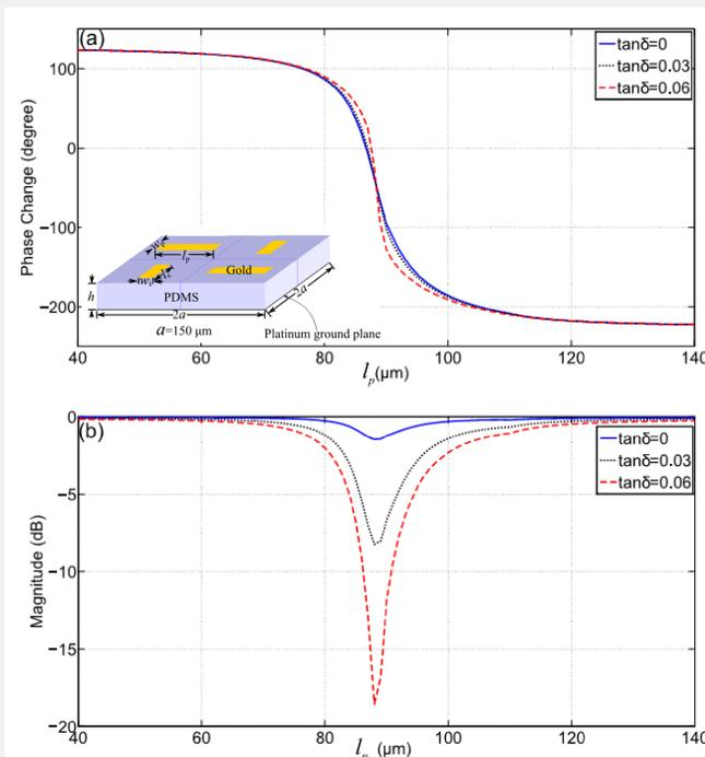
Simulated reflection coefficients for 2D uniform infinite arrays with different PDMS loss tangent.
