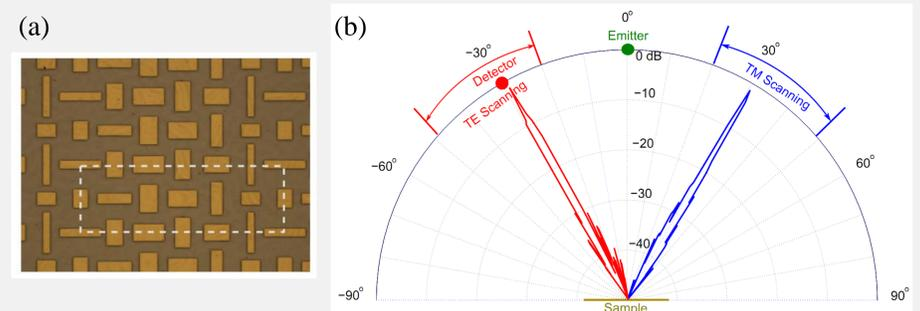
(a) Microscopy image for a small part of the reflectarray. (b) Measured radiation patterns for the TE (red line) and TM (blue line) polarizations of the reflectarray. The normal incident wave can be efficiently deflected into two different directions with the properties of polarization dependence.
