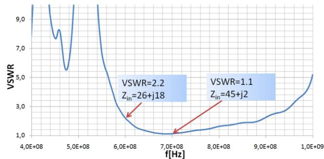
Fig.6. Measured VSWR and  $Z_{in}$  with ARC
