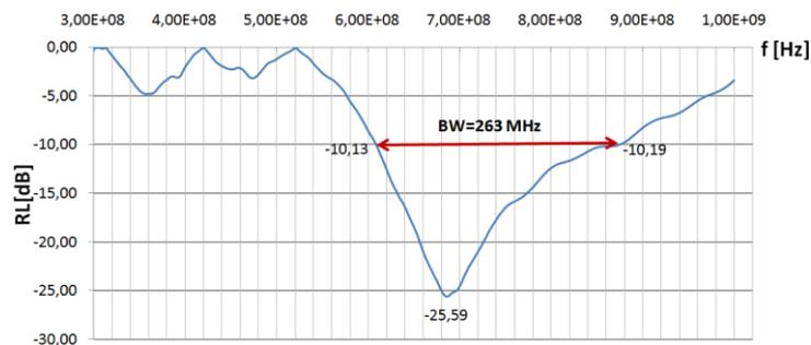
Fig.7. Bandwidth determination for ARC
