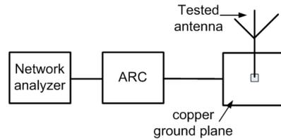
Fig.4. Block diagram of measurement setup
