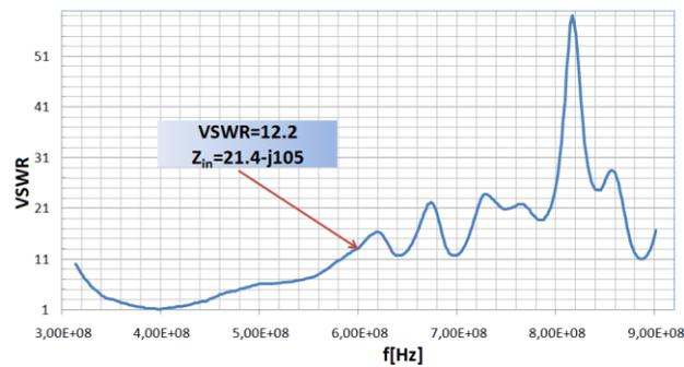
Fig.5. Measured VSWR and  $Z_{in}$  without matching
