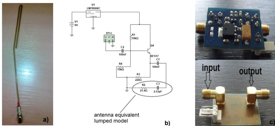
Fig.3. ARC design: a) ESA used in the investigation, b) ARC scheme, c) ARC prototype
