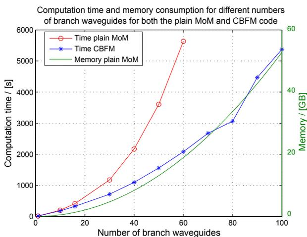
Fig. 4. Total time required by plain MoM and CBFM codes to calculate S-parameters at 5 GHz for waveguide junctions with different numbers of branch waveguides. The CBFM curve represents the worst case, i.e., no CBFs were reused in different slots. Memory requirement is only shown for plain MoM. According to Eqs. (8), the memory compression factor is 2500 in this case.
