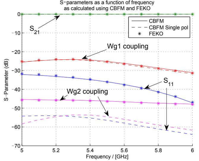
Fig. 3. S-parameters as a function of frequency for a waveguide junction consisting of a feed waveguide connected to two branch waveguides through weakly excited slots, as calculated by three different methods.
