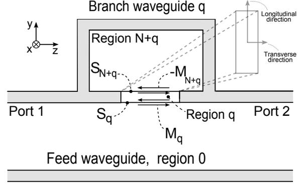
Fig. 2. Cross section showing feed waveguide and branch waveguide number  $q$ , together with a labeling of apertures, magnetic currents and canonical regions.
