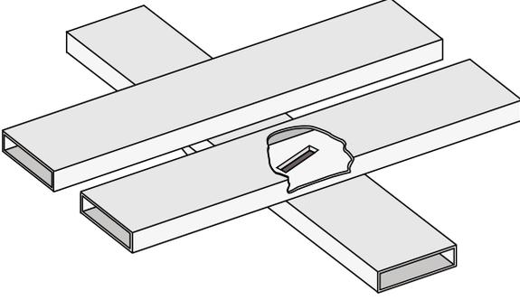
Fig. 1. Waveguide coupling junction with two branch waveguides. One branch waveguide has been cut open to show the slot connecting it to the feed waveguide below.
