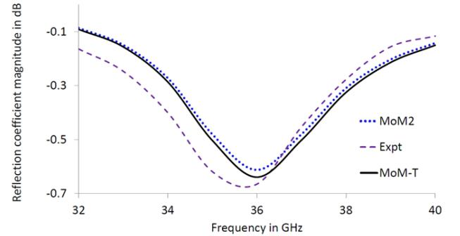
Fig. 3 Computed and measured values of the reflection coefficient magnitude for normal incidence (Case A).
