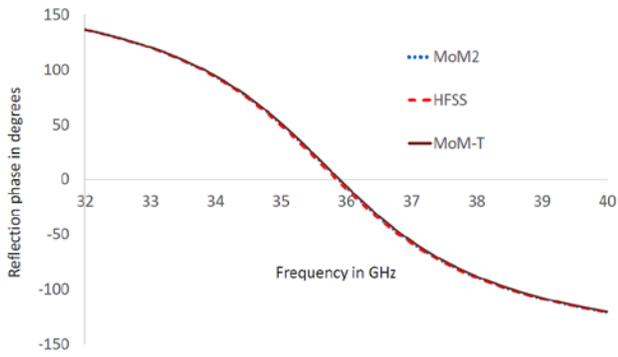
Fig. 7 The reflection coefficient phase for a reflectarray with a superstrate at normal incidence.
