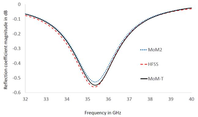
Fig. 10 The reflection coefficient magnitude for a reflectarray with a superstrate for TM polarization at  $45^\circ$ .
