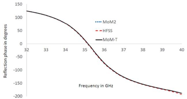
Fig. 11 The reflection coefficient phase for a reflectarray with a superstrate for TM polarization at  $45^\circ$ .
