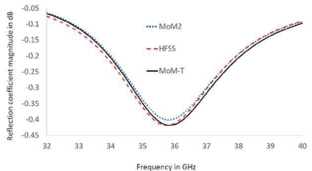
Fig. 6 The reflection coefficient magnitude for a reflectarray with a superstrate at normal incidence.
