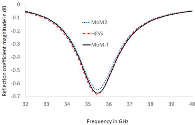
Fig. 8 The reflection coefficient magnitude for a reflectarray with a superstrate for TE polarization at  $45^\circ$ .
