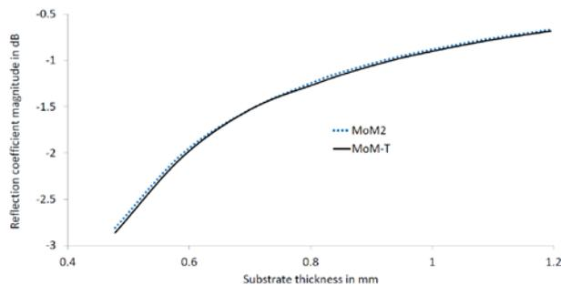
Fig. 5 The reflection coefficient magnitude versus substrate thickness for Ku band.
