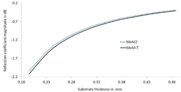
Fig. 4 The reflection coefficient magnitude versus substrate thickness for Ka band.
