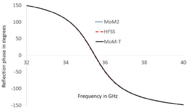
Fig. 9 The reflection coefficient phase for a reflectarray with a superstrate for TE polarization at  $45^\circ$ .
