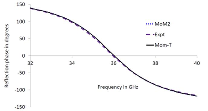
Fig. 2 Computed and measured values of the reflection coefficient phase for normal incidence.
