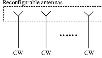
Fig. 2. Active DM transmitter with reconfigurable array elements
