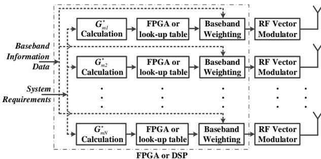
Fig. 4. Generic digital DM transmitter architecture [17].
