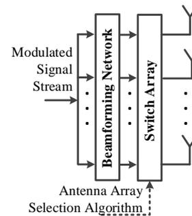
Fig. 6. Structure of ASM or 4-D antenna array.
