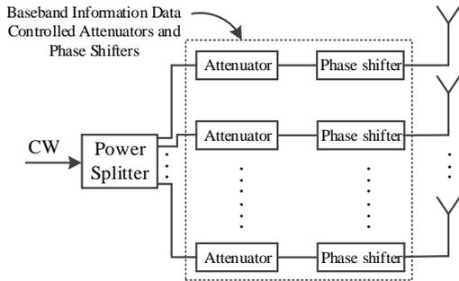
Fig. 3. Generic excitation-reconfigurable DM transmitter array [11].
