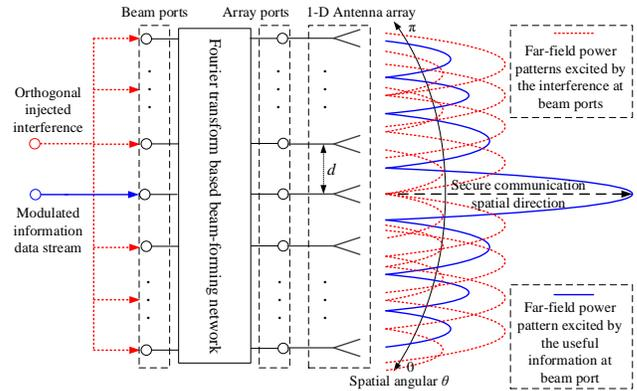
Fig. 5. Fourier beamforming network enabled DM transmitters [32].
