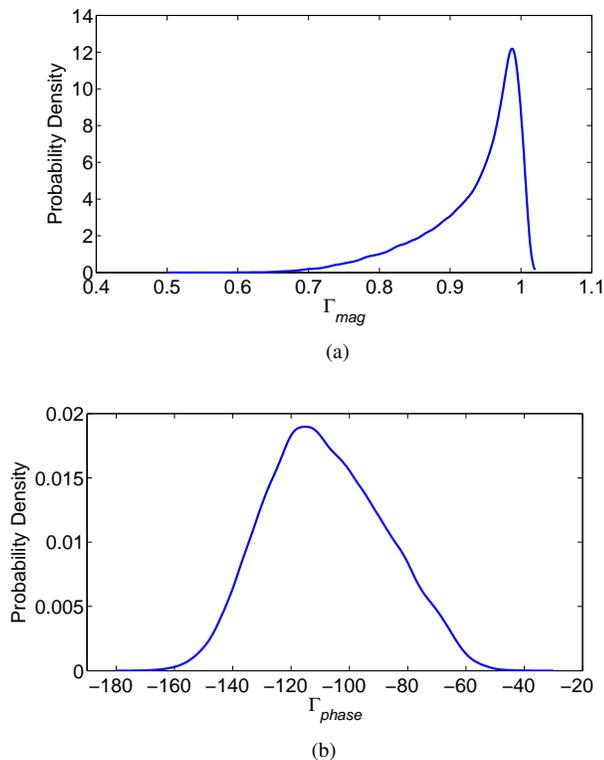
Fig. 2. Probability Density as functions of (a) Magnitude of Reflection Coefficient and (b) Phase of Reflection Coefficient
