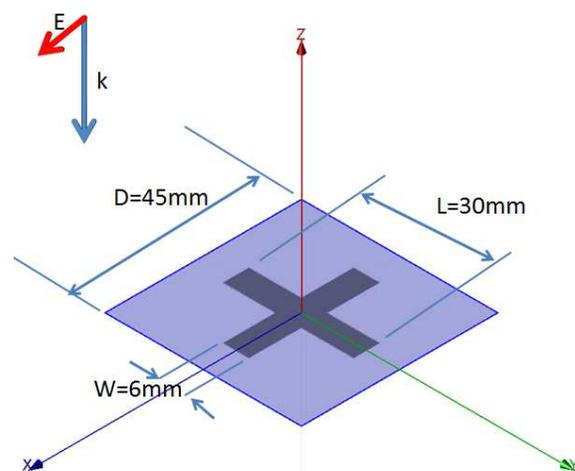
Fig. 1. The input parameters of cross-dipole FSS element
