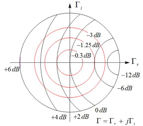
Fig. 15. Load reflection coefficient plane: Red circles – Received power relative to maximum, Black circles – Scattered power relative to maximum received power.
