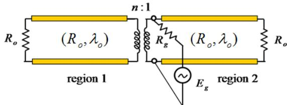
Fig. 24. Ideal transformer transmission line representation for the zero backscatter antenna in the transmit mode.
