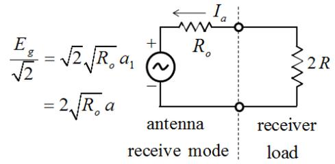
Fig. 9. Conventional Thevenin equivalent circuit for the simple antenna as receiver (Fig. 6) excited by an incident plane wave as in Fig. 2.
