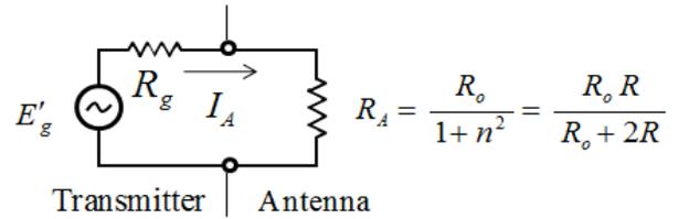
Fig. 25. Standard equivalent circuit for the zero backscatter antenna transmit mode; note  $R_A = R_{TH}$ .
