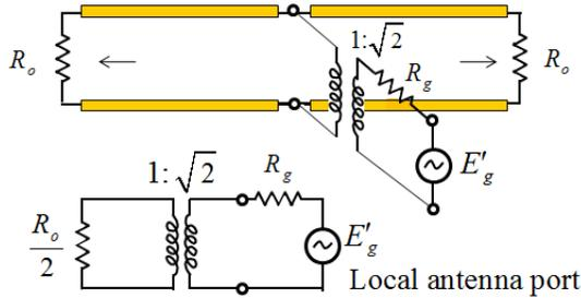
Fig. 10. Transmit antenna transmission line model.
