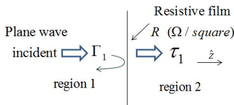
Fig. 1. A 1-dimensional antenna terminated in a plane, infinite resistive film load.
