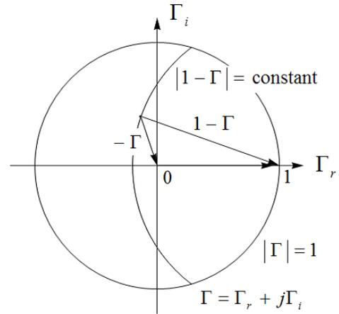
Fig. 16. Construction for scattered power loci (circular arcs) on the complex load reflection coefficient plane.
