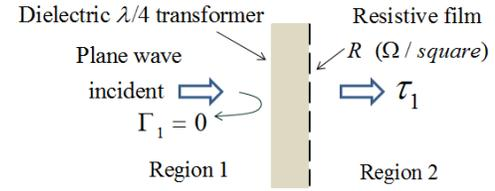
Fig. 19. Resistive film with a quarter-wave dielectric slab.
