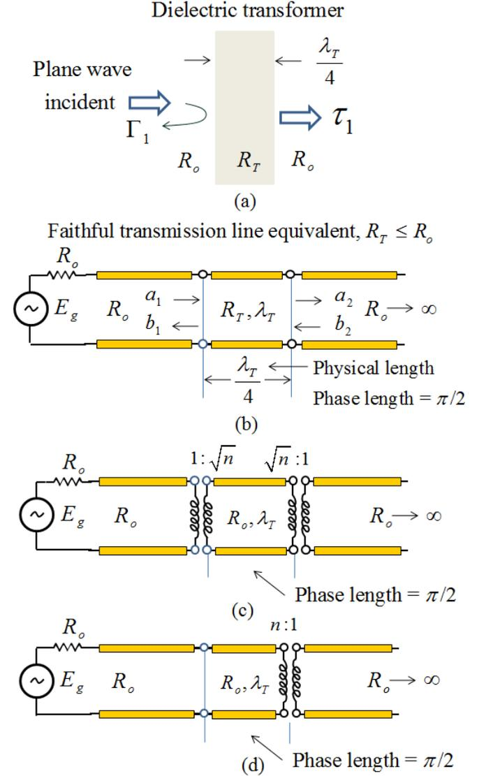
Fig. C1. Quarter wave dielectric slab (remaining when zero backscatter antenna is open-circuited, i. e., resistive film load removed) and equivalent circuit representations: a) Physical structure, b) Faithful transmission line circuit representation, c) Symmetrical ideal transformer equivalent circuit, d) Ideal transformer equivalent circuit.
