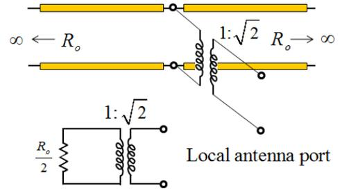
Fig. 18. Transformer necessary to yield matched CMS antenna.
