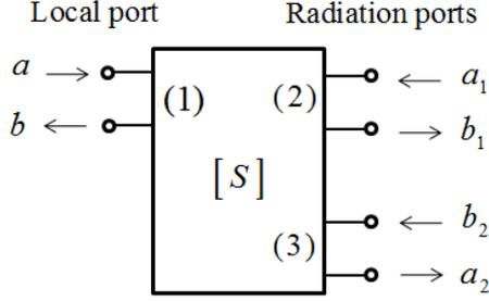
Fig. 17. Scattering matrix of a 1-dimensional antenna.
