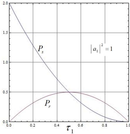
Fig. 4. Received power,  $P_r$ , and scattered power,  $P_s$ , versus transmission coefficient,  $\tau_1$ .
