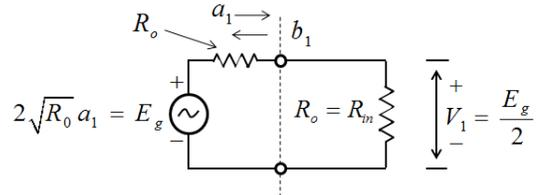
Fig. 22. Equivalent circuit at the input to the transformer when the transformer turns ratio  $n$  is chosen to produce a matched load.
