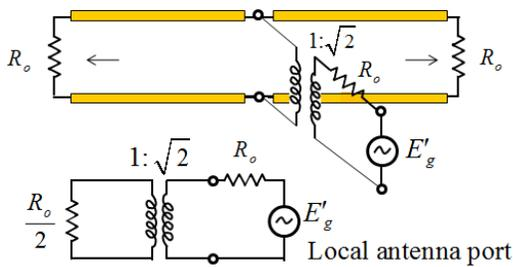
Fig. 7. The simple antenna as transmitter (excited by generator).
