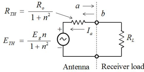
Fig. 21. Standard receive antenna Thevenin equivalent circuit of the zero backscatter antenna.
