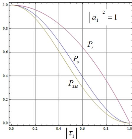
Fig. 23. Plot of normalized powers for the family of reflectionless antennas: received power  $P_r$ , scattered power  $P_s$ , and power apparently dissipated in the Thevenin equivalent impedance  $R_{TH} = R_A$  of the standard receive circuit  $P_{TH}$ .
