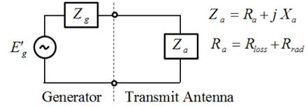
Fig. 5. Antenna as transmitter (excited by generator).
