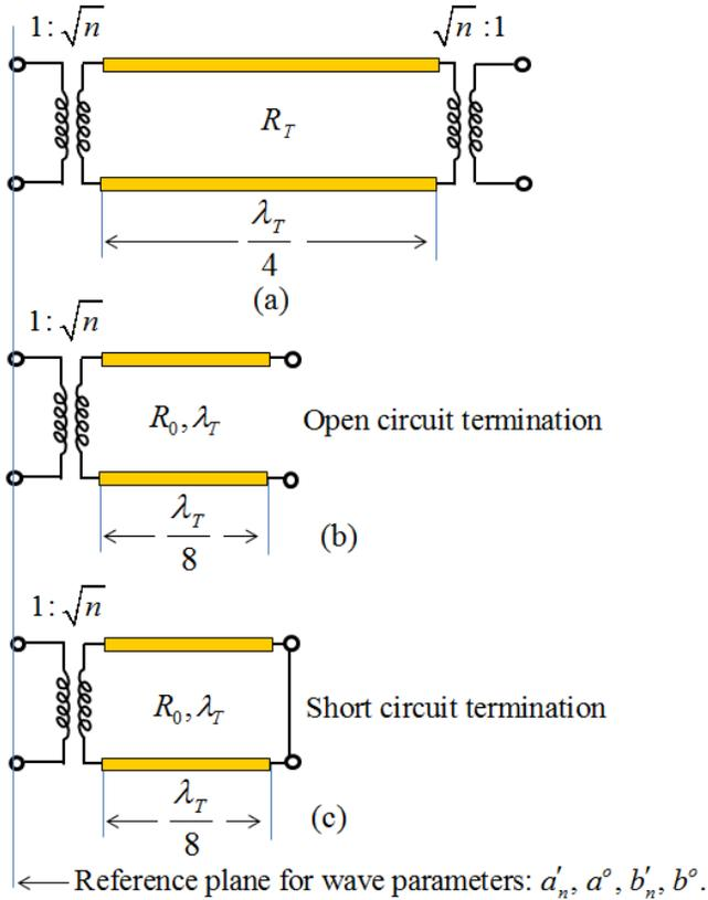
Fig. C2. Circuits for alternative modes eq. C17 incidence calculation: a) Symmetrical ideal former equivalent circuit for quarter wave dielectric slab, b)  $a'_1$  mode incidence – open circuit bisection, c)  $a'_2$  mode incidence – short circuit bisection.
