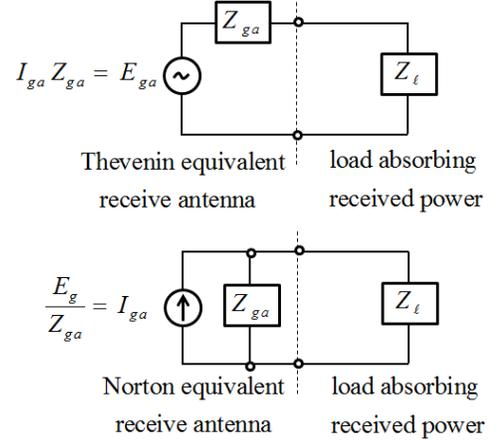
Fig. 6. Thevenin and Norton equivalent receive antenna circuits.
