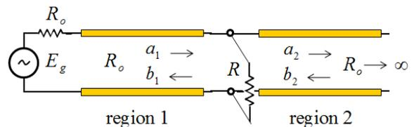
Fig. 2. Transmission line circuit representation, showing an ideal shunt-T load connection.
