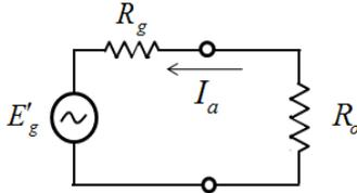
Fig. 11. Circuit representation of the transmit antenna.
