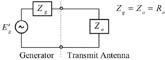
Fig. 8. Conventional equivalent circuit for simple antenna as transmitter (excited by generator).
