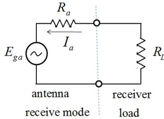
Fig. 12. Thevenin equivalent circuit for a receive antenna.
