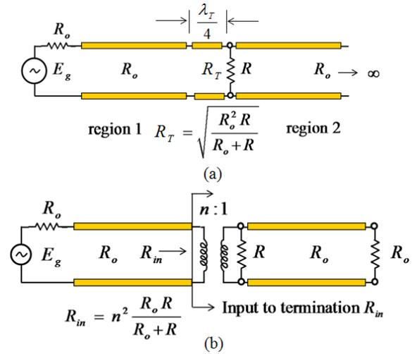
Fig. 20. Circuit models for the zero backscatter antennas - quarter-wave slab transformer with resistive sheet load: a) Faithful transmission line equivalent circuit representation, and b) Ideal transformer equivalent circuit.
