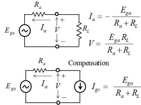
Fig. 13. Compensation theorem applied within the Thevenin equivalent circuit for a receiving antenna.
