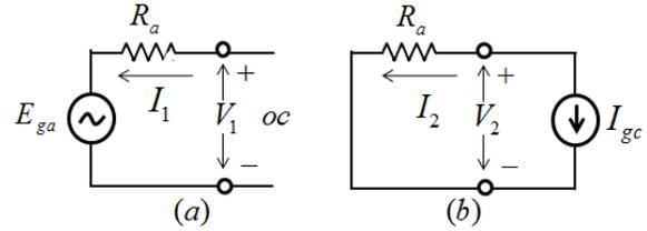
Fig. 14. Principle of superposition of excitations applied to analyze circuit of Fig. 13 into two separate circuits.
