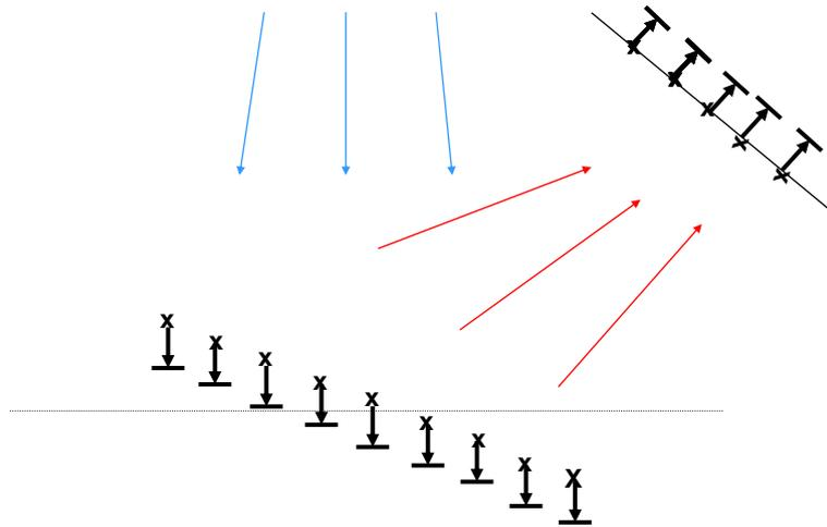
Figure 2. Visual sketch of the rectenna. Each element of the array is indicated by a cross and is loaded with a rectifying circuit. The array elements, originally located over the horizontal line, have been vertically translated and aligned along an inclined line, so that a linear phase difference is induced along the array. Accordingly, the backscattered field can be conveniently directed, and the re-radiated power can be collected.
