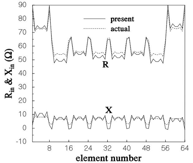
Fig. 8 Effective impedance of 8x8-element array using the 4x4-element array. The dotted curves are the actual impedances from the full wave analysis (WIPL-D).
