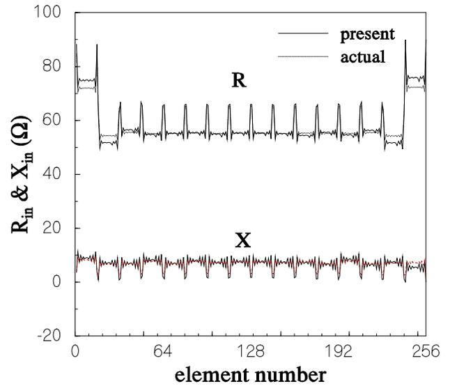
Fig. 12 Effective impedance of  $16 \times 16$ -element array using the  $8 \times 8$ -element array.
