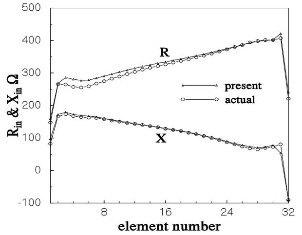
Fig. 21 Effective input impedance of an E-plane linear array of 32 elements with Taylor distribution and -30 DB sidelobe level and scanning at  $45^\circ$  compared with the actual array results.
