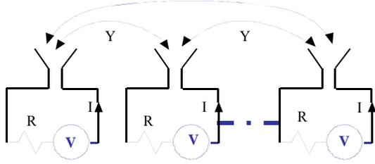
Fig. 1 Equivalent circuit of an antenna array
