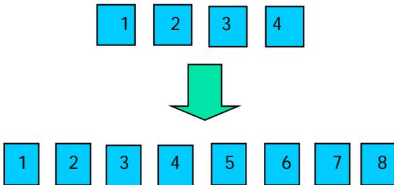
Fig. 3. Linear array of 4 elements that is used to construct a linear array of 8-elements.
