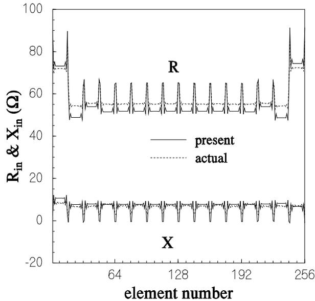
Fig. 10 Effective impedance of  $16 \times 16$ -element array using the  $4 \times 4$ -element array.
