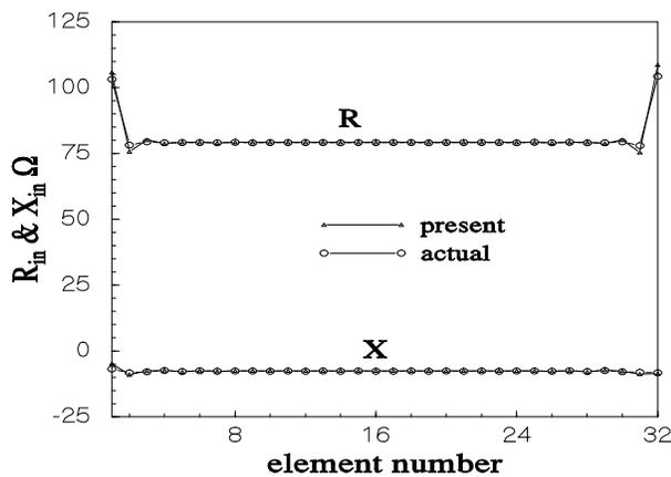
Fig. 15 Effective input impedance of an H-plane 32-element linear array with uniform distribution obtained from 8-element array and compared with the actual array.
