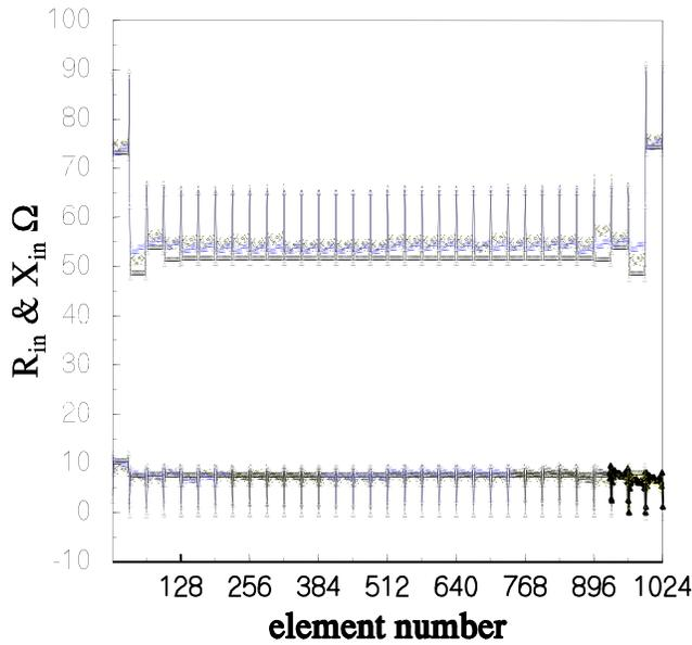
Fig. 14 Effective impedance of 32x32-element array using 4x4 (black), 8x8 (yellow), and 16x16-element array (blue).
