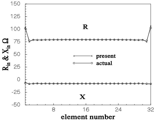
Fig. 19 Effective input impedance of an E-plane linear array of 32 elements with Taylor distribution of -30dB sidelobe level compared with the actual array results.
