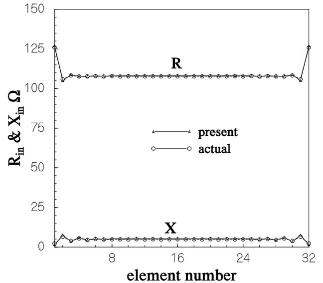
Fig. 16 Effective input impedance of an E-plane linear array of 32 elements with uniform distribution obtained from 8-element array and compared with the actual array.
