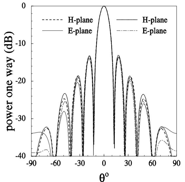
Fig. 9 Radiation patterns of the 8x8-element array. The solid and dashed lines are for the MoM code.
