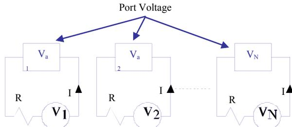
Fig. 2 Equivalent circuit for the effective voltages of the antenna array.
