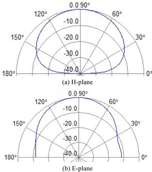
Fig. 7 Radiation patterns of the patch at 4.5 GHz.
