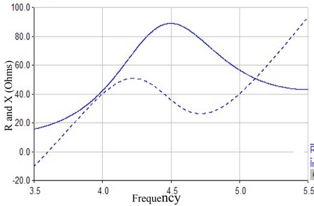
Fig. 6 Input Impedance of the rectangular patch
