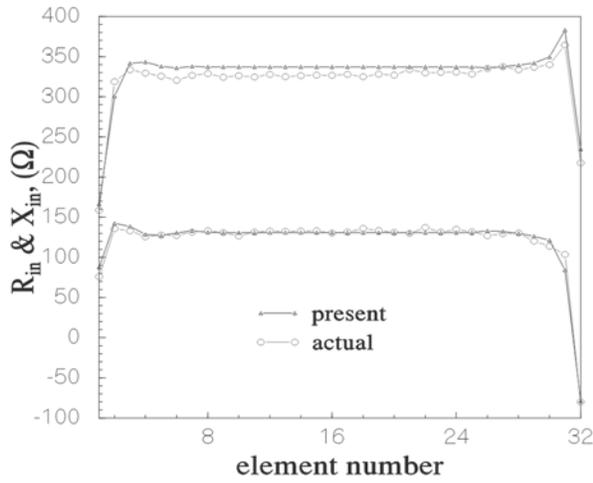
Fig. 18 Effective input impedance of an E-plane linear array of 32 elements with uniform distribution and scanning at  $45^\circ$  and compared with the actual array results.
