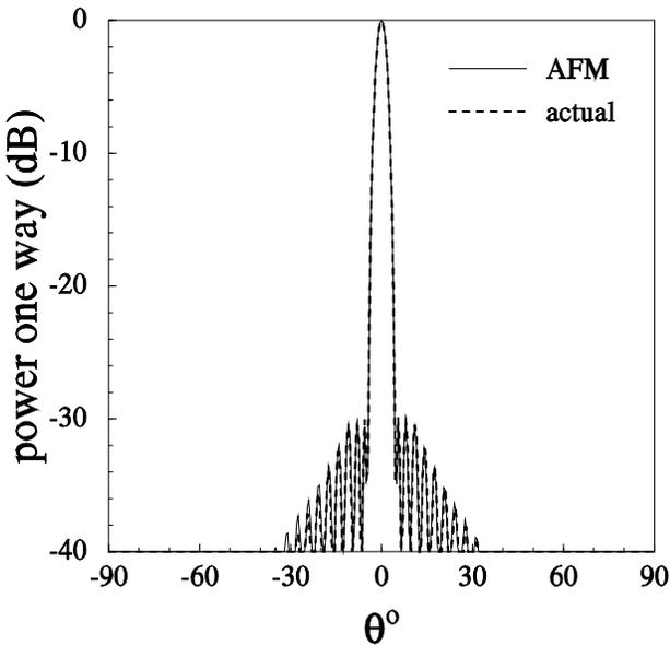
Fig. 20 Radiation patterns of the array in 19.
