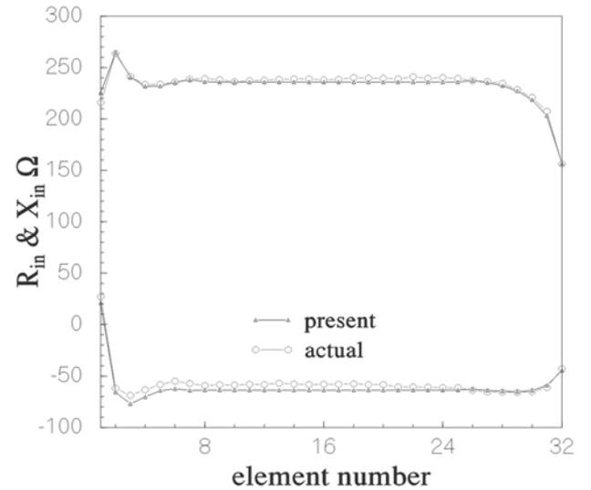
Fig. 17 Effective input impedance of an H-plane linear array of 32 elements with uniform distribution and scanning at 45° and compared with the actual array results.
