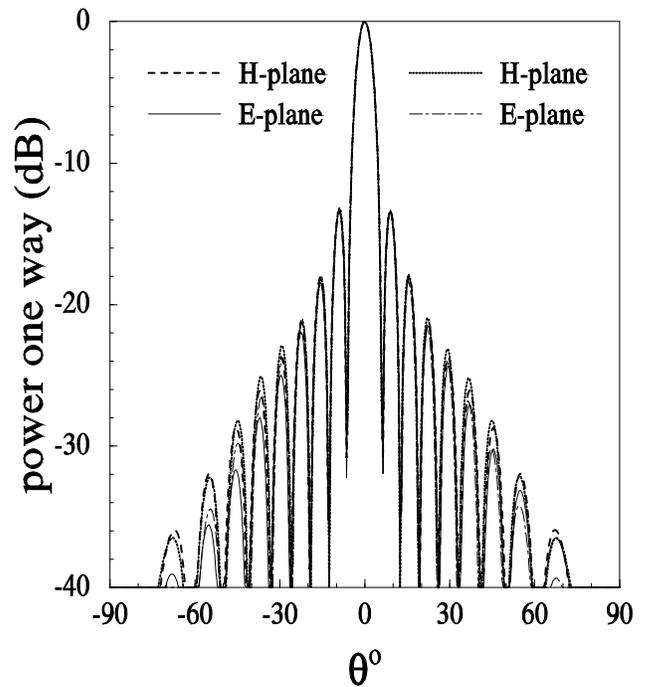
Fig. 13 Radiation patterns of the  $16 \times 16$ -element array using  $8 \times 8$ -element array.
