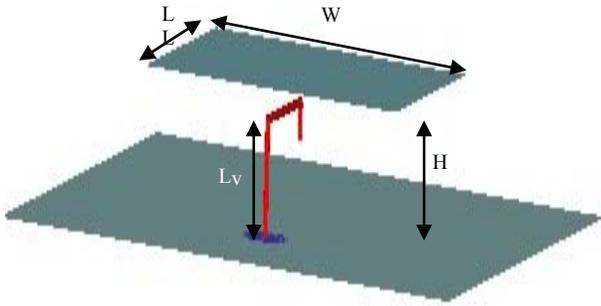
Fig. 5 Geometry of a rectangular patch excited by a Hook-shaped probe.
