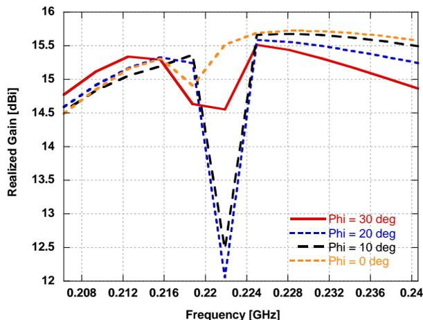
Fig. 17 – Realized gains of the original array for the four different directions.
