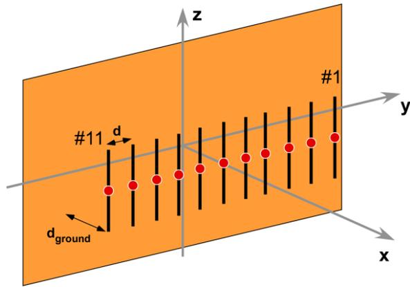
Fig. 12 – Test case #2: array of eleven equally-spaced dipole antennas placed parallel to a finite ground plane.
