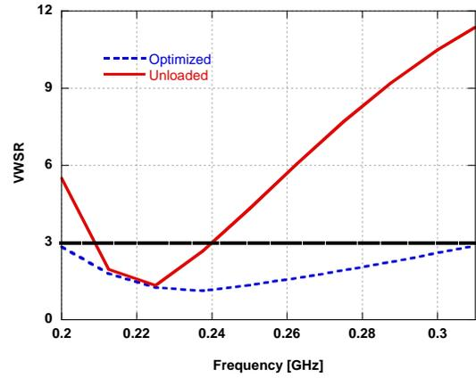
Fig. 10 – Comparison between the original unloaded dipole and the optimized loaded one.
