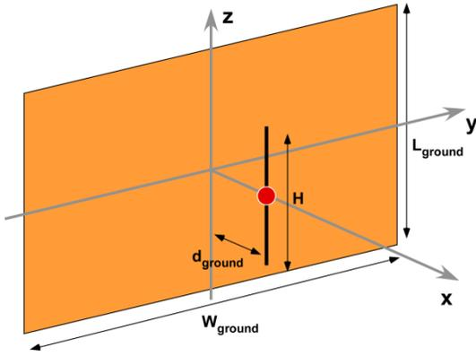
Fig. 9 – Test case #1: dipole antenna placed parallel to a finite ground plane.
