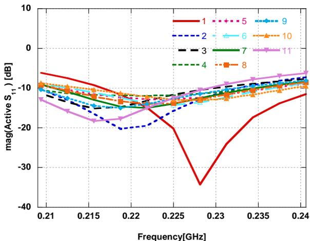
Fig. 16 – Optimized active reflection coefficient for  $\phi_4 = 30$  deg.
