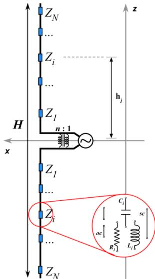
Fig. 7 – Arbitrary loaded dipole antenna with symmetrical  $Z_i$  circuits (series RLC, parallel RLC circuits, open and short circuits).
