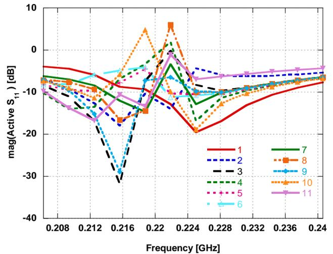
Fig. 14 – Active reflection coefficient for  $\phi_4 = 30$  deg.
