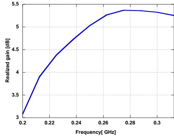
Fig. 11 – Realized gain of the optimized loaded antenna.
