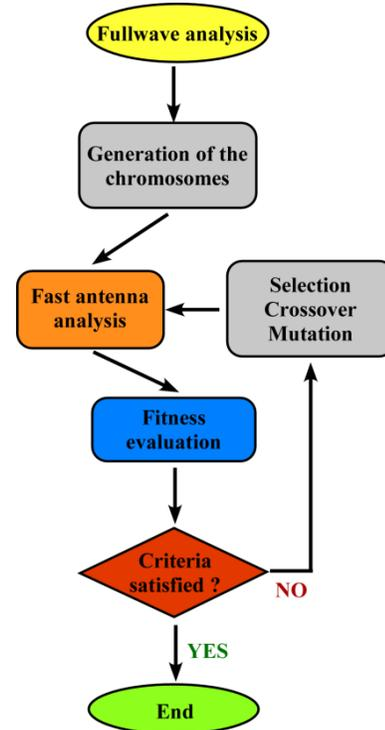
Fig. 8 – Flow chart of the proposed optimization procedure. The full wave solver is employed only once at the beginning of the process.
