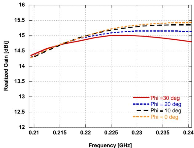
Fig. 18 – Realized gains of the optimized array for the four different directions.
