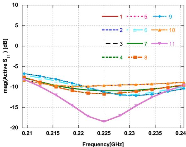
Fig. 15 – Optimized active reflection coefficient for  $\phi_1 = 0$  deg.
